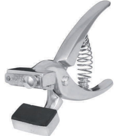
MI-01-1022 Small Tattoo Pliers Light weight pattern, designed for small animals. Made of aluminum alloy. Head holds four dies, for a total of four digits. Size 0.25".
